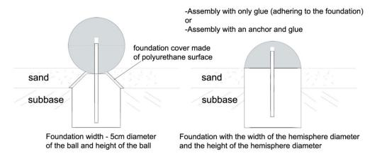
Note: The delivery includes a sphere/hemisphere (optional steel anchor and glue). Standalone installation is expected.
