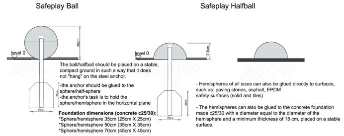
The drawing shows the method of assembling a sphere/hemisphere with a concrete foundation and an anchored steel pipe \*applies to a sphere/hemisphere with a diameter of 35cm (foundation 25cm x 25cm)
