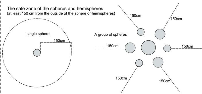
Note: The product can be placed in various configurations, when a group of several pieces is placed next to each other and their HIC <= 150 cm, the zone is 150 cm and is always determined from the extreme part of the sphere or hemisphere.
